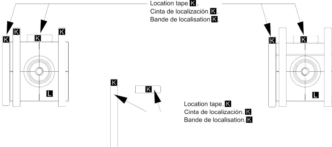
Remove the pedestals **L** / **X** keeping the location tape **K** in place.
