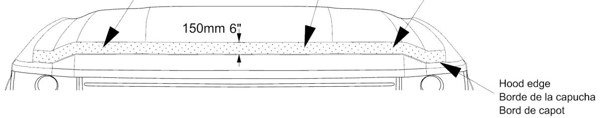
Using one of the surface wipes **B** provided and clean the first 150mm of front of the hood.
