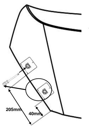
8. The positions of the pedestals are shown in **illustration**. Use the corner of the pedestal for the measurements. The pedestals should have an even 2mm gap from the edge of the hood to the bottom edge of the pedestal
