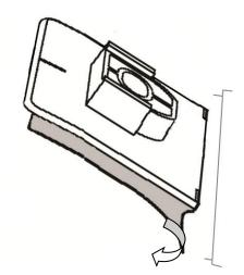
13. Remove the protective backing from the adhesive on the pedestals and install on the hood surface.
