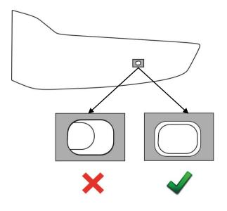
10. Confirm correct positioning of the pedestals, by adjusting the pedestal position on the hood to align with the holes in the hood protector.
