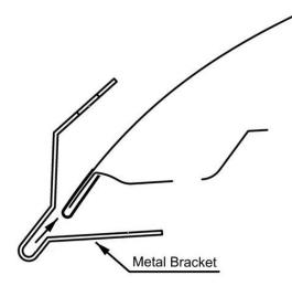
4. Install Metal Brackets over the hood edge in their correct positions. Align the hole in the bottom leg of the bracket with the round hole in the hood. See *Illustration*.
