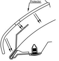
10. Confirm correct positioning of the pedestals, by adjusting the pedestal position on the hood to align with the holes in the hood protector.
