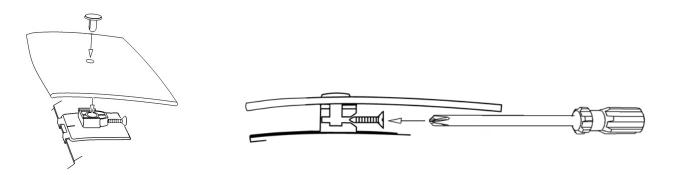
18. On some vehicles <u>it may be necessary to adjust</u> the hood bumpers and/or latch for proper clearance. Note: Do not pull on the protector when opening or closing the hood.
