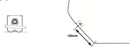
9. Place the protector temporarily onto the metal brackets aligning the holes in the protector with the holes in the metal brackets. This step will allow you to confirm the position of the adhesive pedestals.
