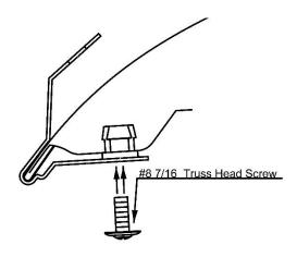
8. Insert the #8 x 7/16" truss head screw through the metal bracket "B" and into the expansion plug. Tighten the screw into the expansion plug making sure the leg of the bracket is well seated against the surface of the hood. See Illustration.
