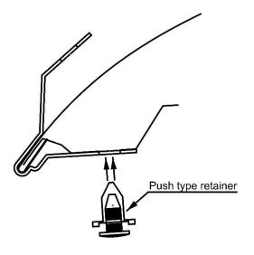
6. Insert a push type retainer through the metal bracket "A" and into the hood. Ensure leg of the bracket is well seated against the surface of the hood and push the center pin of the retainer assembly to lock it into place. See Illustration.
