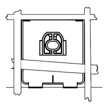
14. Remove the hood protector, and outline the perimeter of the pedestals with masking tap or the repositionable tape strips supplied to help final installation.
