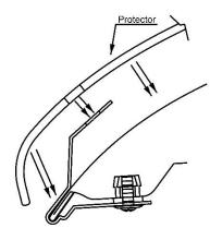
11. Place the protector temporarily onto the metal brackets aligning the holes in the protector with the holes in the metal brackets. This step will allow you to confirm the position of the adhesive pedestals.
