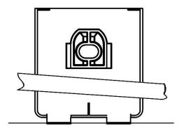
9. Dry fit the adhesive pedestals using masking tape or the repositionable tape strips supplied to hold them in position.
