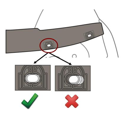
13. Confirm correct positioning of the pedestals, by adjusting the pedestal position on the hood to align with the holes in the hood protector.
