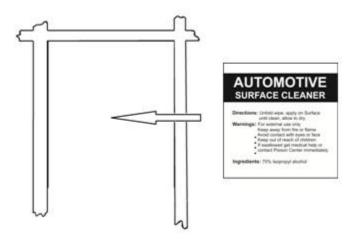
15. Remove the pedestals and thoroughly clean the outlined area with the alcohol wiping pad. This will insure all wax, finger prints and oils are removed from the hood surface in the bonding area. Wipe dry with a soft cloth or paper towel.
