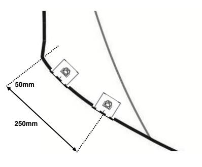
10. The positions of the pedestals are shown in illustration. Use the center mark on the leading edge of the pedestal for accurate measuring. The fingers incorporated on the leading edge of the pedestal will help ensure the correct position relative to the hood edge. When correctly positioned the fingers should contact the leading edge of the hood.
