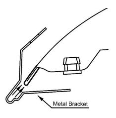
Install the metal brackets "B" at the correct location over the hood edge, aligning the hole in the bottom leg of the bracket with the hole in the expansion plug.
