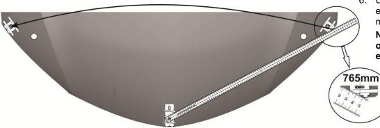
Use the center mark on the leading edge of the pedestals for accurate measuring.
