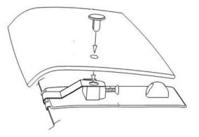
14. At the three (3) large pedestal locations drop a pin through the protector and into the pedestal
