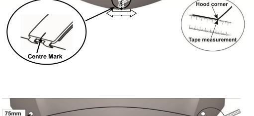
Install the two (2) bumpons as shown. <u>Attention: Bumpons must be installed</u> <u>on the hood, not on the deflector!!!</u> If the bumpons are installed on the deflector, they may wear through the paint.
