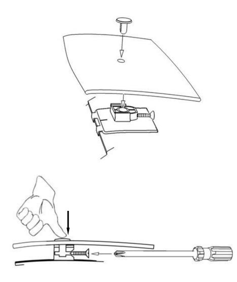
16. At the four (4) small pedestals, drop a pin through the protector and into the pedestal.
