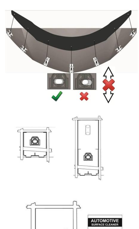
7. Place the hood protector on the pedestals to confirm proper positioning, make any necessary adjustments.
