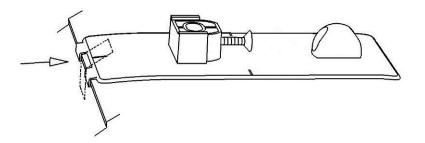
12. For the large adhesive pedestals above the grill, peel and fold an antiabrasion film pad in half over the hood edge between the fingers on each pedestal.
