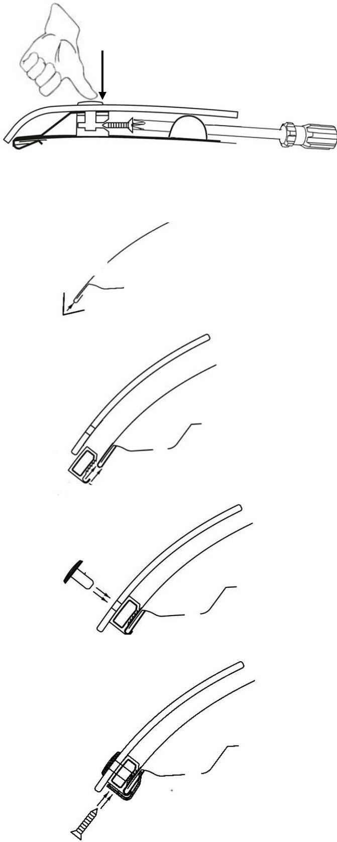
14. Maintain slight pressure on the pin, to ensure proper seating of the components, while simultaneously tightening the screw on all of the adhesive pedestals.
