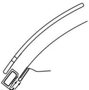
13. Place a clip body over each of the anti-abrasion film pads on the edge of the hood.
