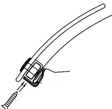
15. Insert a screw through an 'L'- bracket and into the clip body.
