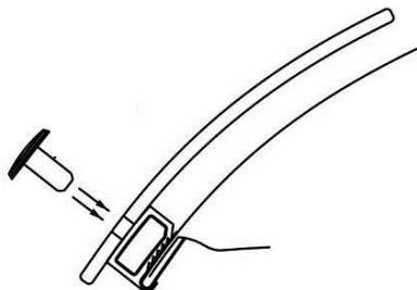
14. Insert a pin through the protector into each of the clip bodies.
