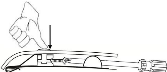
8. Remove the protective backing film from each of the adhesive pedestals and install them on the hood surface.
