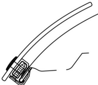
15. Peel and fold the four (4) large anti-abrasion film pads in half over the hood edge aligned with the outer holes of the deflector in the area above the headlights.
