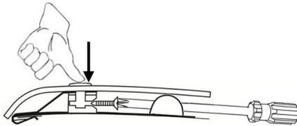
10. Peel and fold the anti-abrasion pads in half over the hood edge between the fingers on the pedestals.
