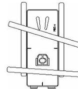
The positions of the pedestals are shown in the **illustrations**. Use the center mark on the leading edge of the pedestals for accurate measuring. The fingers incorporated on the leading edge of the pedestal will help ensure the correct position relative to the hood edge. When correctly positioned the fingers should contact the leading edge of the hood.
