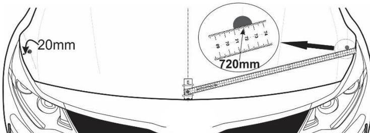
**\* Tape measure is always located below the measuring point**
