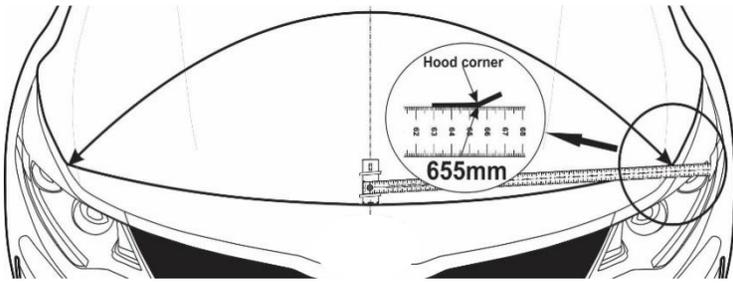
**Locate center pedestal using installation tape measure.**
