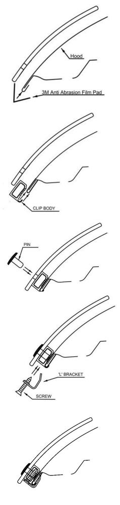
14. Peel and fold the four (4) large anti-abrasion film pads in half over the hood edge aligned with the outer holes of the deflector in the area above the headlights.
