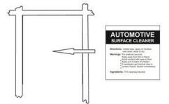
Remove the pedestals and thoroughly clean the outlined area with the alcohol wiping pad. This will insure all wax, finger prints and oils are removed from the hood surface in the bonding area.
