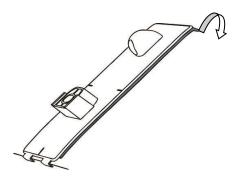
Remove the protective backing film from each of the adhesive pedestals and install them on the hood surface.
