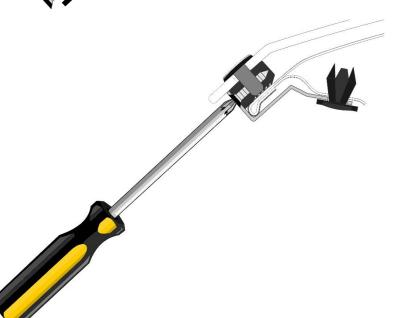
10. Ensure all metal brackets and clip bodies are properly aligned and tighten the screws into each of the three clip bodies. Note the orientation of the metal brackets. They should be perpendicular to the hood edge. See illustration.
