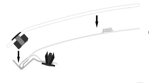
8. With all three pins and clips bodies in place, lower the hood protector onto the hood and align the holes in the 3 metal brackets with the holes in the clip bodies.
