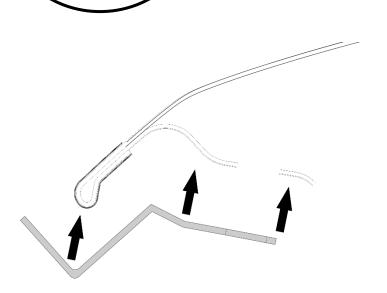
4. One at a time, place the metal bracket over the hood edge in their correct positions. Align the hole in the bottom leg of the bracket with the round hole in
