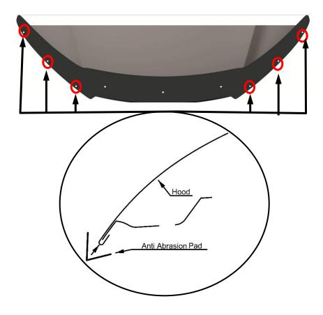
8. Peel and fold the anti-abrasion pads in half over the edge of the hood in line with the three holes in the protector over each of the headlights. See Illustration. Repeat for remaining push-type retainers.
