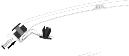
9. Insert a #6 x 5/8" screw through the metal bracket and into each clip body.
