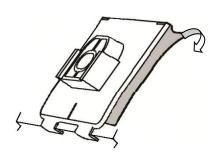
Remove the protective backing from the adhesive on the pedestals and install on the hood surface.
