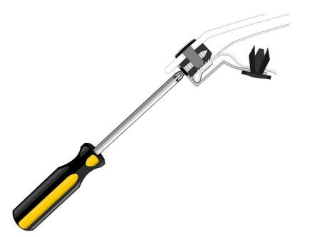
12. Ensure all metal brackets and clip bodies are properly aligned and tighten the screws into each of the clip bodies. Note the orientation of the metal brackets. They should be perpendicular to the hood edge. See illustration.
