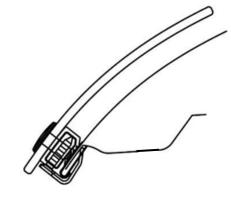
23. Make sure all the components are well seated together; the protector is centered on the hood, and then tighten the screws into the clips.
