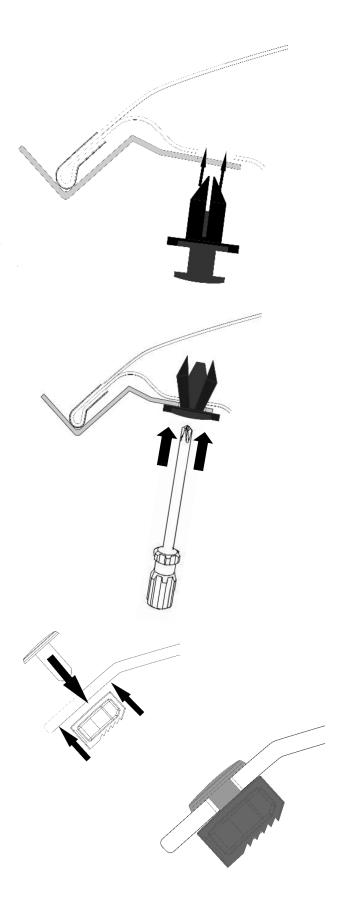
7. Insert a push-type retainer through the metal bracket and into the round hole in the hood. **See Illustration.**
