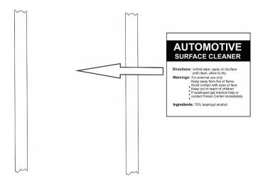
15. Remove the pedestals and thoroughly clean the outlined area with the alcohol wiping pad. This will insure all wax, finger prints and oils are removed from the hood surface in the bonding area.
