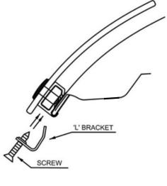
22. Insert a #6 x 5/8" screw through an 'L'- bracket (Type A) and into the clip body.
