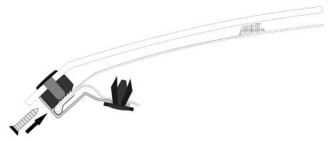
11. Insert a #6 x 5/8" screw through the metal bracket and into each clip body.
