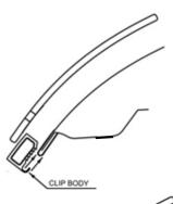
19. Locate the two (2) unused holes in the hood protector. Wrap an anti-abrasion film pad over the hood edge at these locations.
