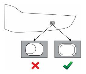
13. Confirm correct positioning of the pedestals, by adjusting the pedestal position on the hood to align with the holes in the hood protector.
