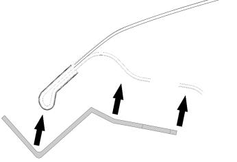
6. Install Type B Metal Brackets over the hood edge in their correct positions.
