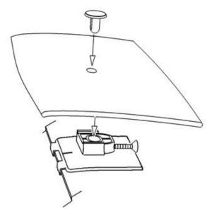
24. At the pedestal locations, drop a pin through the protector and into the pedestal.
