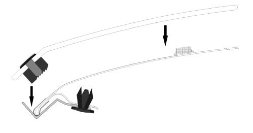
10. With both pins and clips bodies in place, lower the hood protector onto the hood and align the holes in the metal brackets with the holes in the clip bodies.
