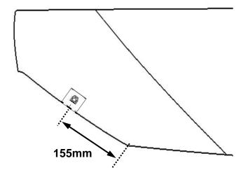
4. The positions of the pedestals are shown in **illustration**. Use the center mark on the leading edge of the pedestal for accurate measuring. The fingers incorporated on the leading edge of the pedestal will help ensure the correct position relative to the hood edge. When correctly positioned the fingers should contact the leading edge of the hood.
