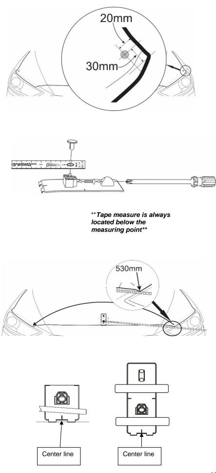
Install the two (2) bumpons as shown. <u>Attention: Bumpons must be installed</u> <u>on the hood, not on the protector!!!</u> If the bumpons are installed on the protector, they may wear through the paint.
