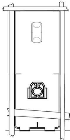
7. Remove the hood deflector, and outline the perimeter of the pedestals with masking tape or the repositionable tape strips supplied to help final installation.
