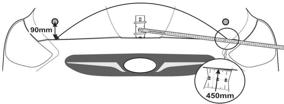
**Locate bump-ons using installation tape.**
