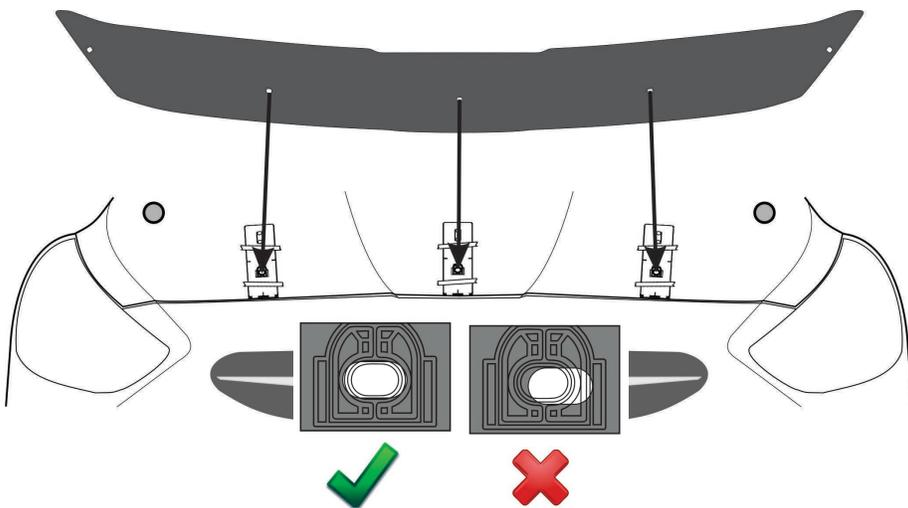
6. Place the hood deflector on the pedestals to confirm proper positioning. Ensure the holes in the deflector align with those in the pedestals. If necessary, reposition the pedestals so all attachment positions are correct and the deflector is well centered.
