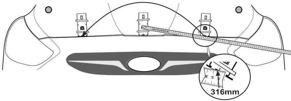
**Locate other pedestals using installation tape.**
