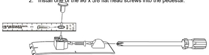
**Locate centre pedestal using installation tape.**
