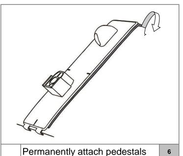
Remove the red backing from the adhesive and install on the hood surface. Tip: Hook the fingers on the pedestals over the hood edge and rotate the unit into position. After installation, remove the tape strips and "wet out" the pedestal base by applying pressure with your thumb around the surface of the
