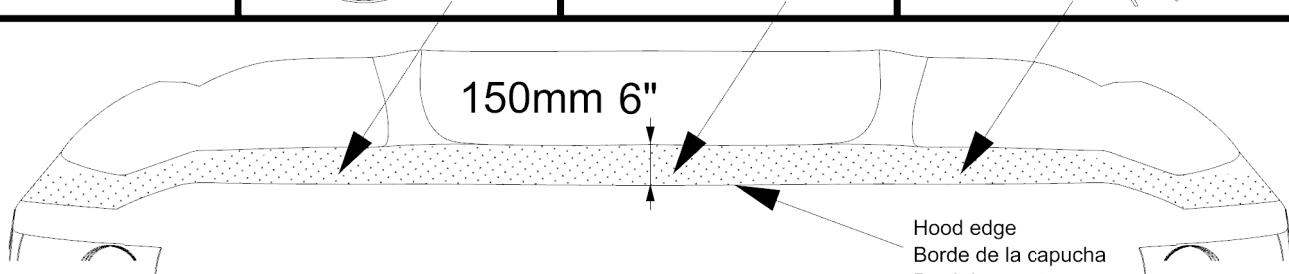
Using one of the surface wipes **B** provided and clean the first 150mm of front of the hood.
