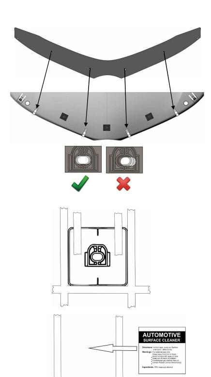
Place the protector temporarily onto the metal brackets, aligning the holes in the protector with the holes in the metal brackets. This step will allow you to check the position of the adhesive pedestals and adjust if necessary.
