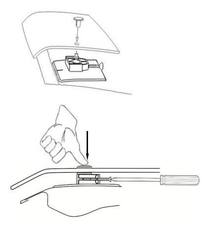
13.Insert a pin through the protector and into each of the two (2) pedestals. Maintain pressure on the head of the pin to ensure the protector is seated against the pedestal and tighten the screw until snug. Do not over-tighten!
