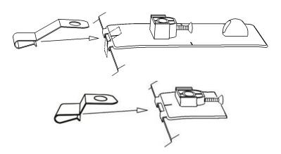
10. Push a metal mounting bracket over the hood edge on top of the anti abrasion pad installed previously. Ensure the bracket is fully engaged over the hood edge and the hole in the bracket is aligned with the hole in the pedestal.
