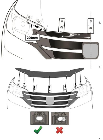
The positions of the pedestals are shown in illustration. Use the center mark on the leading edge of the pedestals for accurate measuring. The fingers incorporated on the leading edge of the pedestal will help ensure the correct position relative to the hood edge. When correctly positioned the fingers should contact the leading edge of the hood.
