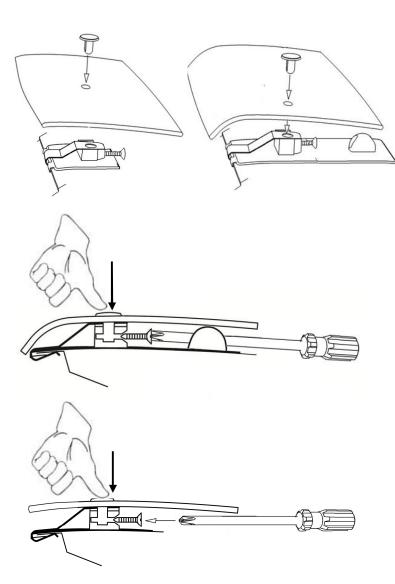
11. Place the hood protector on the pedestals and drop a pin through the protector and into the pedestal. Maintain slight pressure on the pin, to ensure proper seating of the components, while simultaneously tightening the screw. Repeat for remaining pedestal locations.
