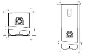
Remove the hood protector, and outline the perimeter of the pedestals with masking tape or the repositionable tape strips supplied to help final installation.
