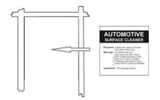
Remove the pedestals and thoroughly clean the outlined area with the alcohol wiping pad. This will insure all wax, finger prints and oils are removed from the hood surface in the bonding area.
