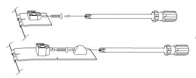
8. Start a #6 x 5/8 flat head screw into each pedestal a few turns. The tip of the screw must not protrude into the hole where the attachment pin will install later.
