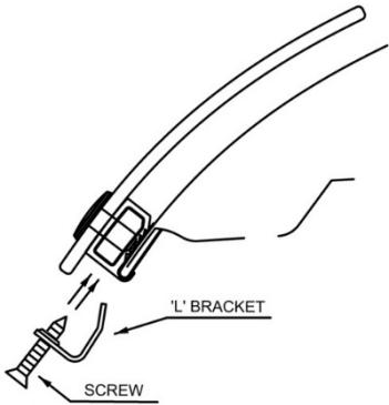
13. Insert a screw through an 'L'- bracket and into the clip body.
