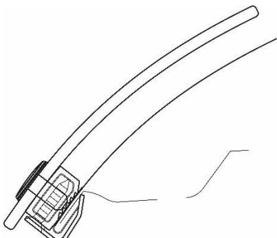
14. Ensure all the components are well seated together and then tighten the screws into the clip bodies.
