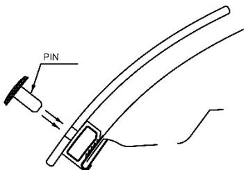
12. Insert a pin through the protector into each of the clip bodies.
