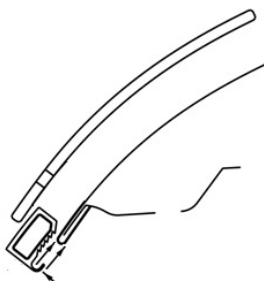
11. Place a clip body over each of the abrasion pads on the edge of the hood.
