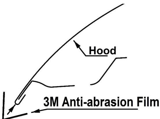
10. Peel and fold the four (4) abrasion film pads in half over the hood edge aligned with the outer holes of the protector in the area above the headlights.
