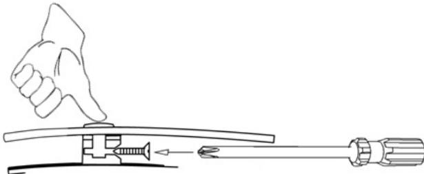
9. Place the protector on the pedestals and, starting at the center location, install a pin through the protector and into the pedestal. Maintain slight pressure on the pin, to ensure proper seating of the components, while simultaneously tightening the screw on each of the adhesive pedestals.
