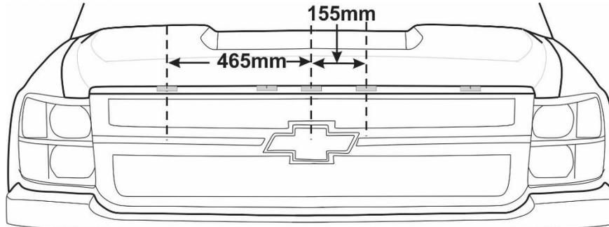
4. Install the square expansion plugs into the top of the adhesive backed pedestals. Use the centering notch on the pedestals to align its location with the pencil mark on the tape from the previous Step. **Note:** When located correctly the leading edge of the pedestal will butt against the back of the grill.
