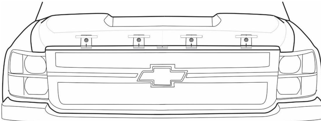
6. Using masking tape or the repositionable tape strips, outline each pedestal as shown. This will aid in placement after cleaning. Remove the pedestals and clean the contact area with the automotive surface cleaner. Dry with a soft cloth or paper towel.
