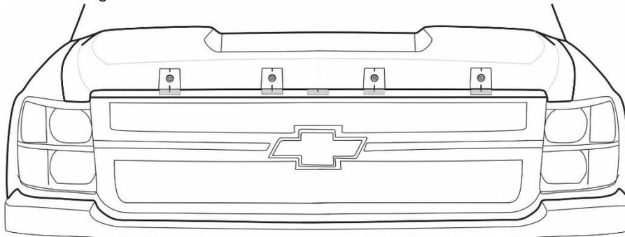
5. Temporarily tape the pedestals to surface of the hood in their determined positions. Confirm correct placement by placing the hood protector on top of the four pedestals. When positioned correctly the four (4) holes in the center area of the protector will align with the holes in the expansion plugs. Adjust if necessary and reconfirm the pedestal locations using the measurements in the illustration and the hood protector.
