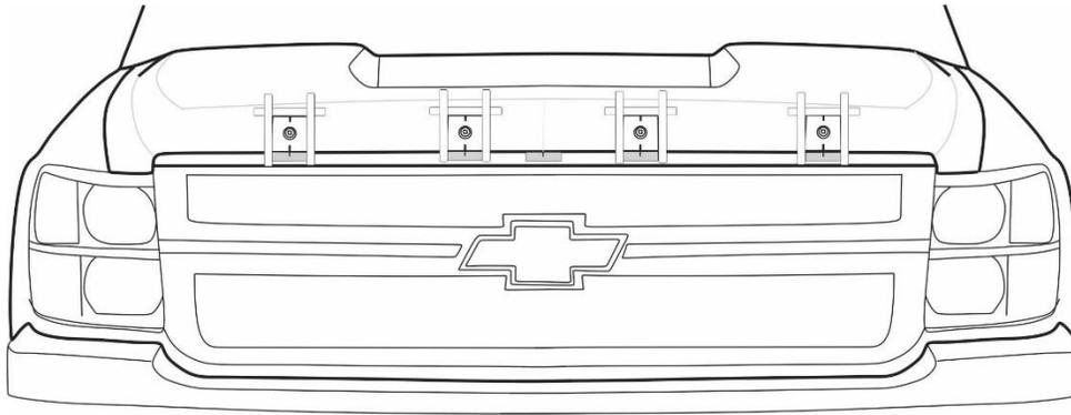
7. Remove the protective film from the bottom of the pedestal and adhere to the hood surface by contacting the leading edge of the pedestal with its location at the back of the grill surround and rotating into place on the hood surface. Wet out surface of the pedestal to ensure complete contact of the adhesive with the surface of the hood. **See Illustration.**
