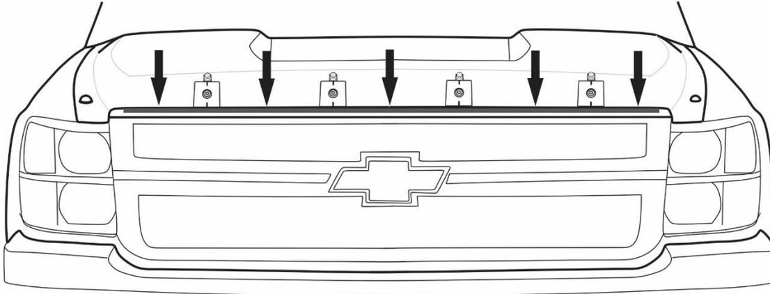
11. Place the hood protector on the hood and fasten the four (4) # 8 x 7/16+wafer head screws through the protector and into the expansion plugs. **Do not over-tighten.**
