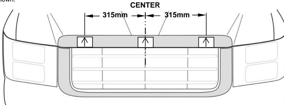
4. Install the square expansion plugs into the top of the adhesive backed pedestals. Use the centering notch on the pedestals to align it's location with the pencil mark on the tape in the previous Step. **Note:** When located correctly the pedestal leading edge will butt against the back of the grill surround at all 3 locations.
