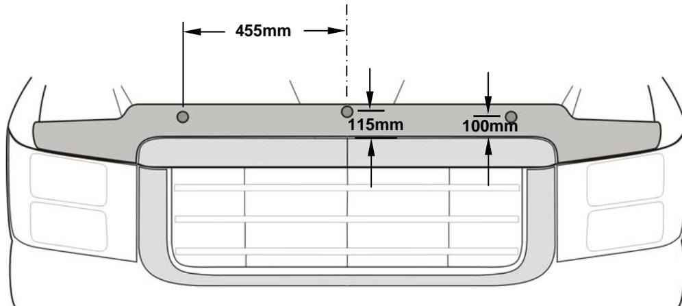
9. Place the hood protector on the hood and fasten the (3) # 8 x 7/16" truss head screws through the protector and into the expansion plugs. **Do not over-tighten.**
