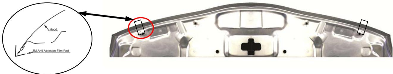
5. Install Metal Brackets over the hood edge in their correct positions. Align the hole in the bottom leg of the bracket with the round hole in the hood.
