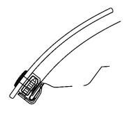
16. Place a clip body over each of the anti-abrasion film pads on the edge of the hood.
